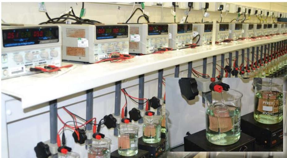
The electrolysis area in full operation (Inset: During electrolysis the copper deposits from the test solution onto a platinum mesh).
